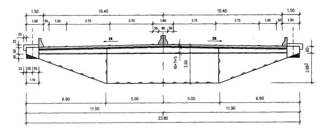
Fig.3 Steel cross section at midspan
