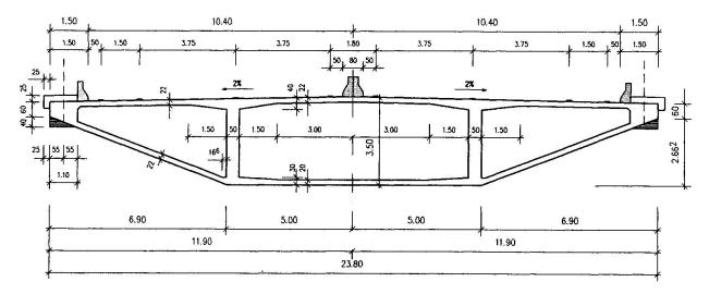
Fig. 2 Concrete cross section at midspan
