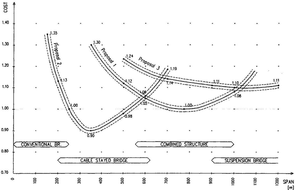
**Fig.5 Relative costs of a bridge with span 300-1000m in Taiwan**
