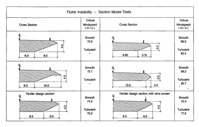
Fig. 8. Sample of investigated box section shapes.
