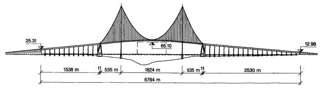
Fig. 2. The East Bridge will carry a 4-lane motorway with two emergency lanes.
