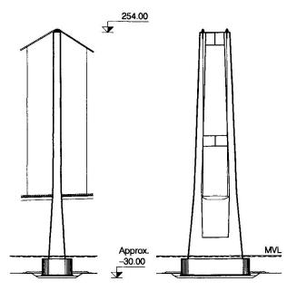
Fig. 11. Concrete pylon layout.
