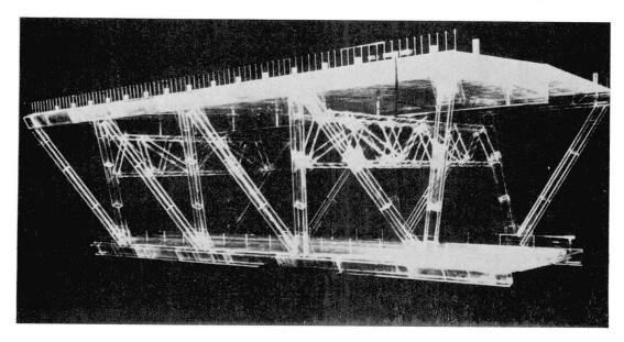
Fig. 4. Model of stiffening beam section
