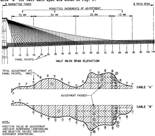
Fig. 2 Adjustment passes. Brooklyn half of Main Span
