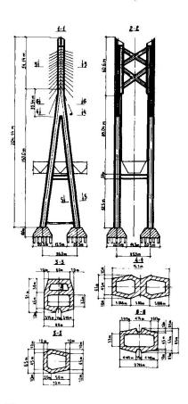
Fig. 2 General view of pylon
