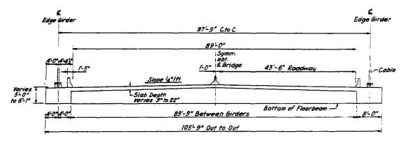
FIGURE 2 - CROSS SECTION
