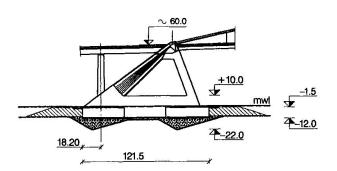
Fig. 12. Anchor block layout.
