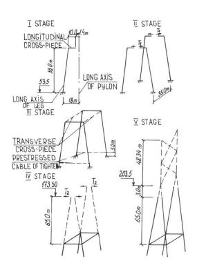
Fig. 3 Pylon erection diagrams
