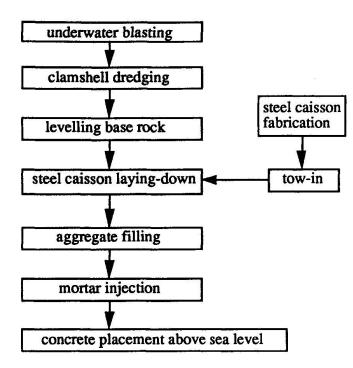
Fig.4 Process of the "laying-down" caisson method
