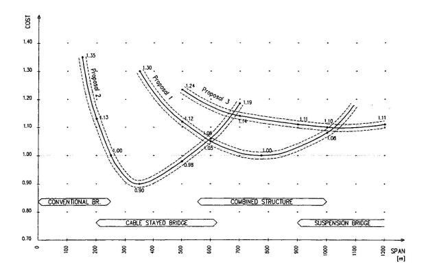
Fig. 5 Relative costs of a bridge with span 300-1000m in Taiwan
