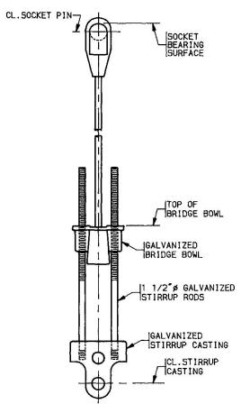
Fig. 1 New wire rope suspender
