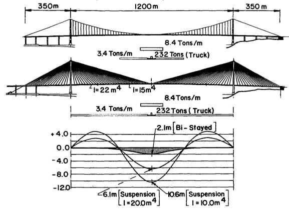
Fig. 6 Comparison of deformational characteristics
