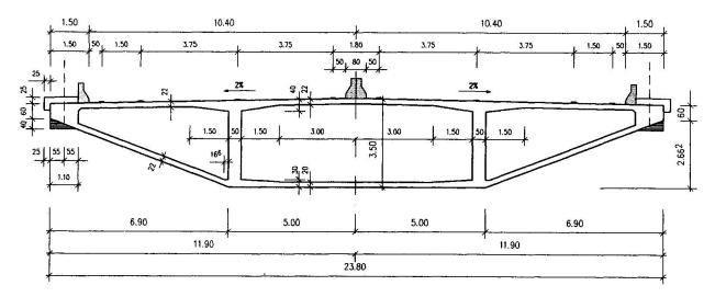
Fig. 2 Concrete cross section at midspan
