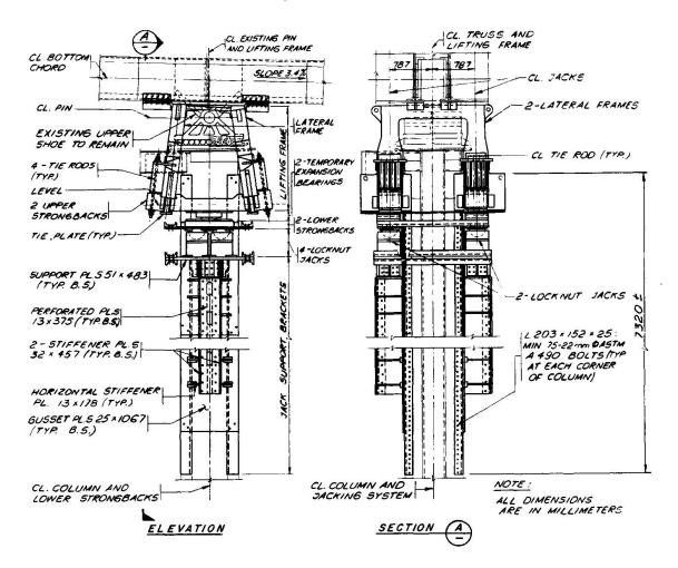
Fig. 4 Bearing replacement jacking system.
