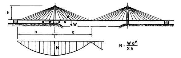
Fig. 1 Generalized cable-stayed bridge schematic
