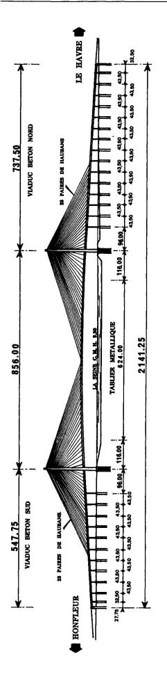
Fig. 3: Longitudinal static configuration of the Normandie Bridge (1989 Projet Détaillé). The central part of the main span, built in steel, is 624-metre long.
