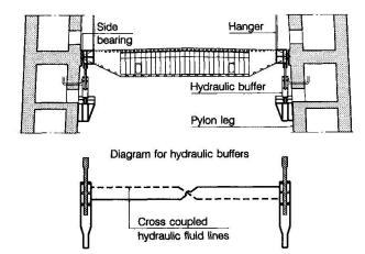
Fig. 9. Arrangement of bridge girder at the pylons.
