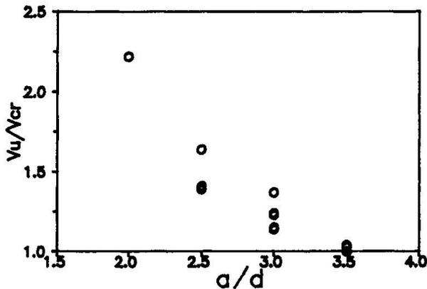
Fig. 2 Measured  $V_u/V_{cr}$  of beams without stirrups
