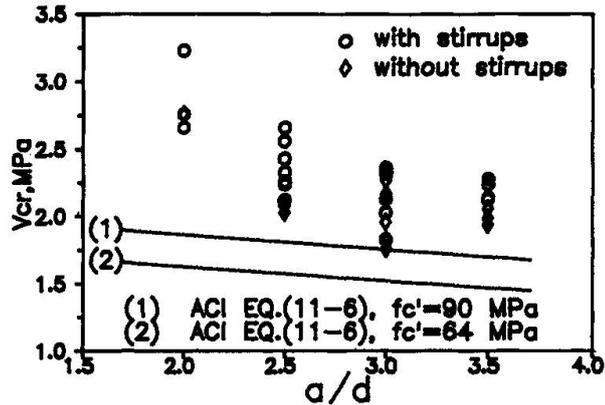
Fig. 3 Comparisons of  $V_{cr}$  measured vs. predicted
