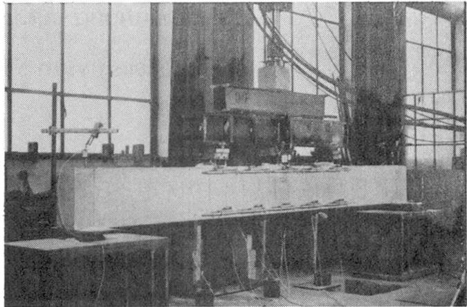
Fig. 1 Testing apparatus for three symmetrical loads
