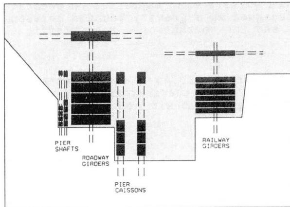
Fig. 3.4 Prefabrication yard.
