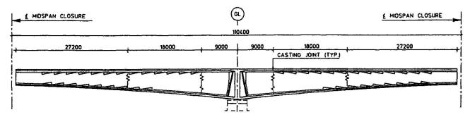
Fig. 3.2 Longitudinal section in bridge superstructure.
