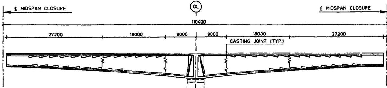
Fig. 3.2 Longitudinal section in bridge superstructure.
