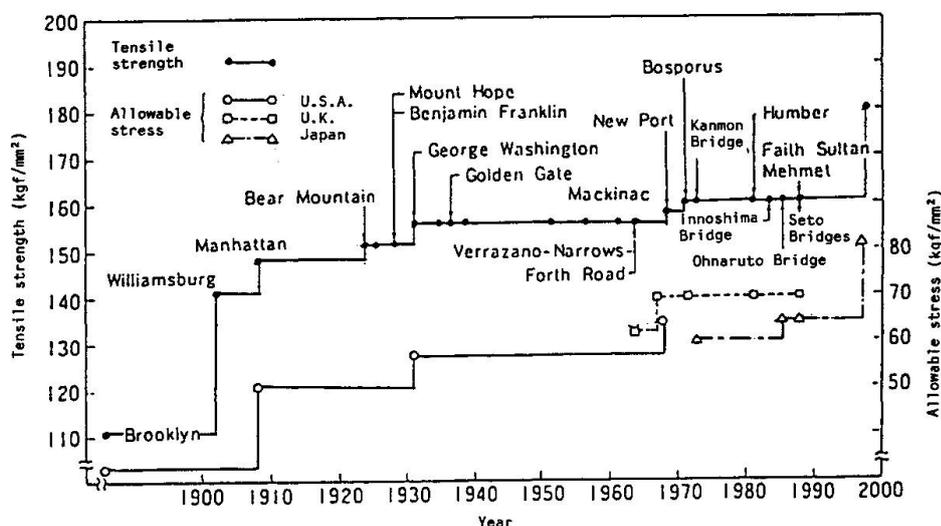
Fig. 1 Improvements in strength of galvanized steel wire
