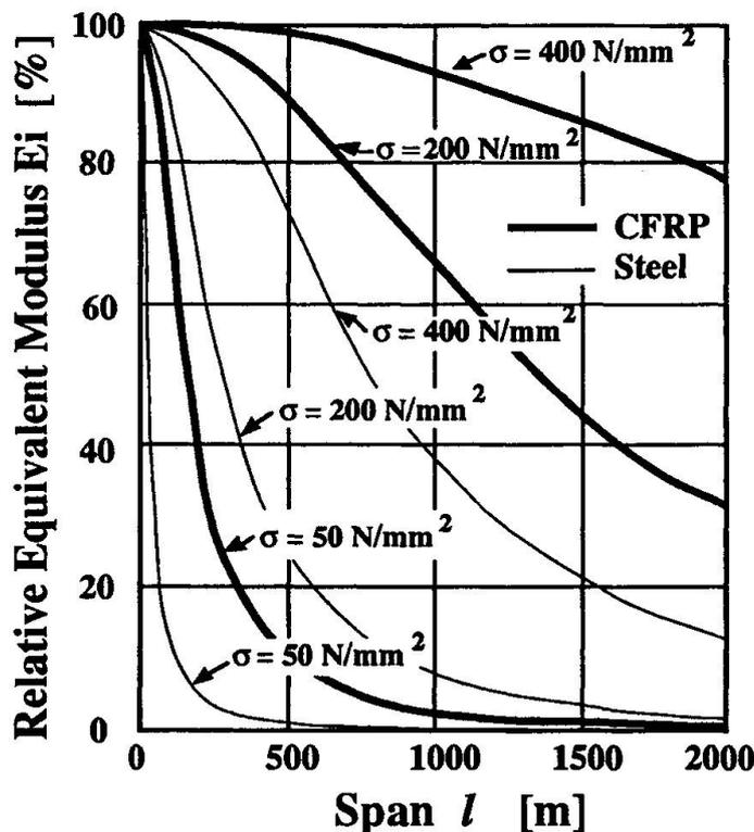
Fig.5 Equivalent modulus vs. span length and pretension
