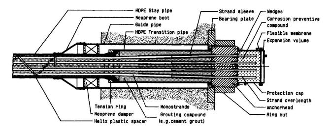
Fig. 2: Cable anchorage
