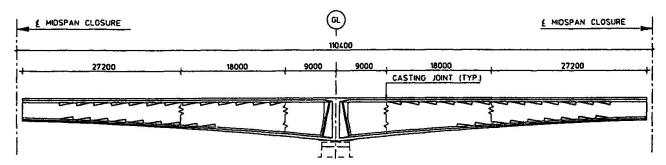
Fig. 3.2 Longitudinal section in bridge superstructure.
