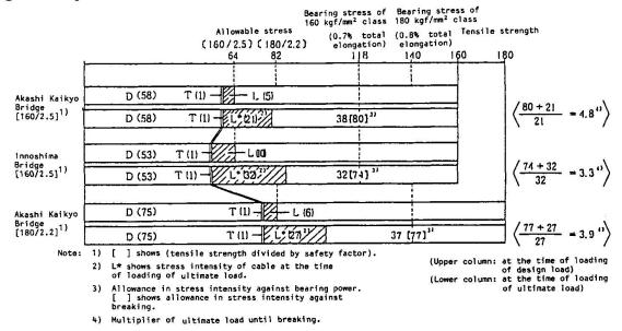
Fig. 4 Cable stress when loaded with the ultimate load (unit: kgf/mm<sup>2</sup>)
