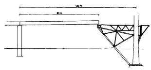
Fig. 2.3 A steel bracket was a support point for a 80 m section.
