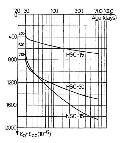
Fig. 3 Experimental initial shorting  $\epsilon_0$  and creep deformation  $\epsilon_{cc}$
