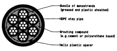
Fig. 1 Cable cross-section
