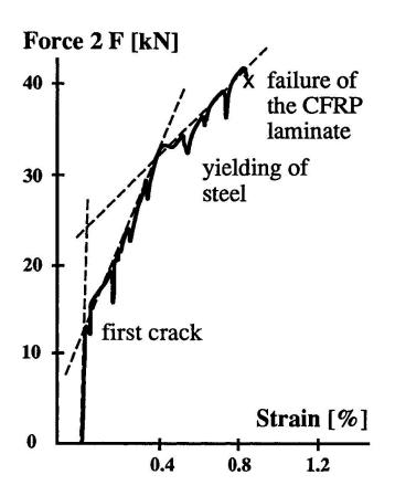
Fig.3 Force vs. strain diagram for a beam with 2.0 m span and strengthened with an 0.3 mm thick CFRP laminate. The force F is given for each loading point, i.e. total load = 2F. The strain was measured in the center of the beam on the CFRP laminate.
