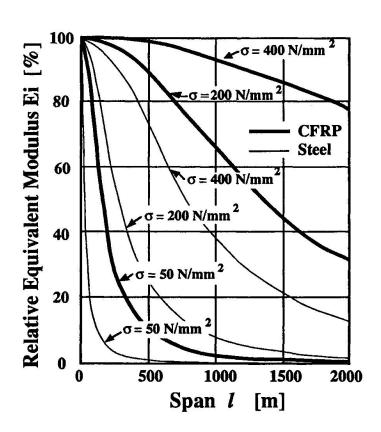
Fig.5 Equivalent modulus vs. span length and pretension
