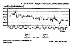
detailled construction control programme for these defined. bridges was Deflections, strains temperatures as also creep and shrinkage effects were recorded and typical results are shown. Porto Novo Bridge deflection of the horizontal of the piers controlled, in order to adjust,
