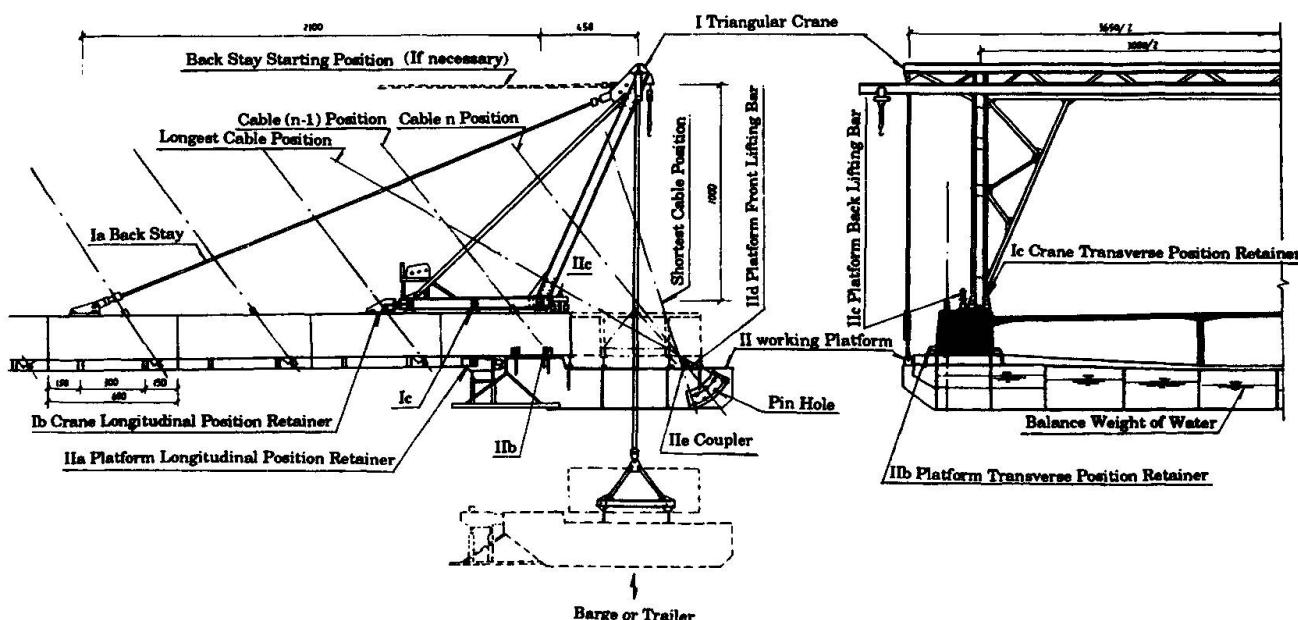
Figure 1. General arrangement of construction equipments
