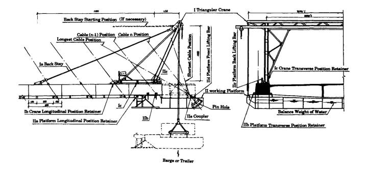
Figure 1. General arrangement of construction equipments
