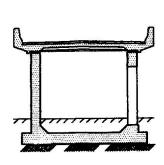
FIG 2: OVERBRIDGE CROSS SECTION
