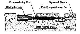
Fig.4 Anchoring device in the beam ( Side view )
