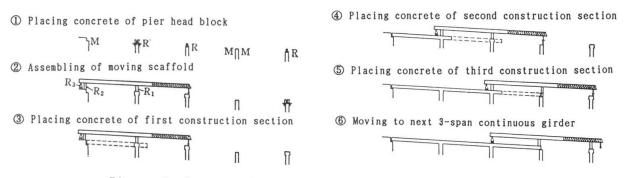
Figure-3 Construction procedure by moving scaffold
