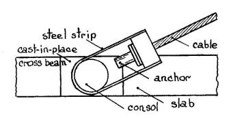
stays are fixed in the saddle -type bearing supports. To fix stays to the stiffening slab cross beams, a new design of the unit (Fig.2) having the of basic advantage unification within the superstructure limits independent of the stays inclination angles, has been developed.
