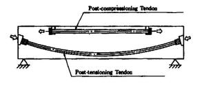
Fig.1 Concept of the bi-prestressing system
