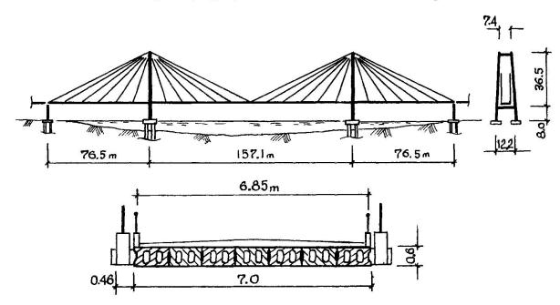
Fig. 1 General view and cross section of cable-stayed bridge
