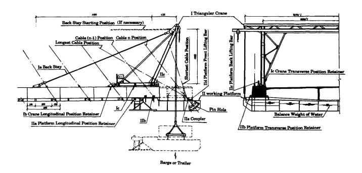
Figure 1. General arrangement of construction equipments
