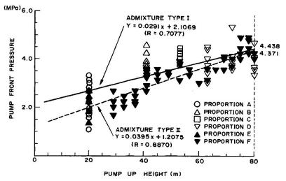
Fig.6 Transition of pump front pressure
