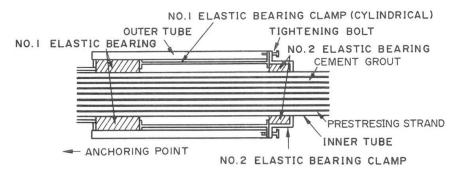
$\underline{\text{Fig.7}}$  Structural details of the elastic bearings for stay cables
