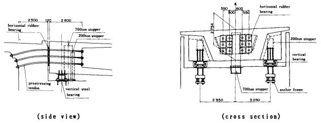
Fig. 5 Bearing at abutment
