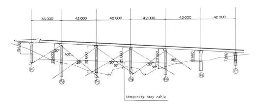
Fig. 6 Temporary stay cable arrangement
