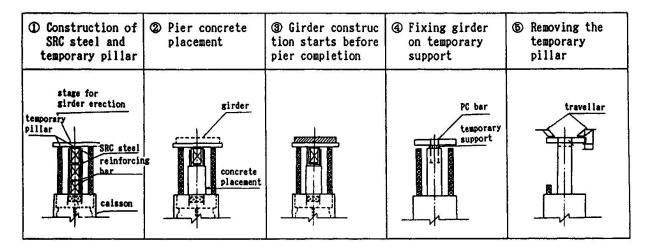
Fig. 4 Pier construction method
