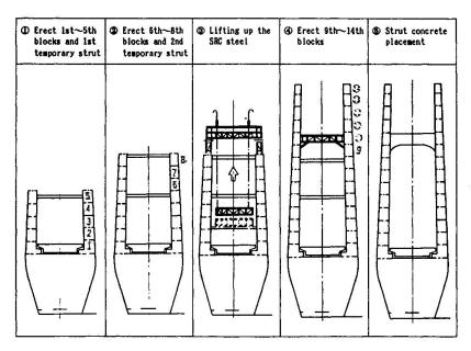
Fig. 5 Tower construction method
