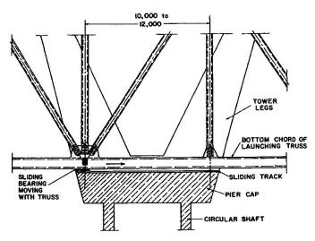
Fig. 3 Truss moving on pier table
