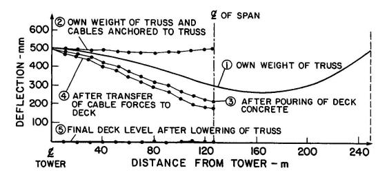
$\frac{\text{Fig.4}}{\text{elevation}}$  Deflections of truss and deck during construction for temporary deck elevation + 500 mm
