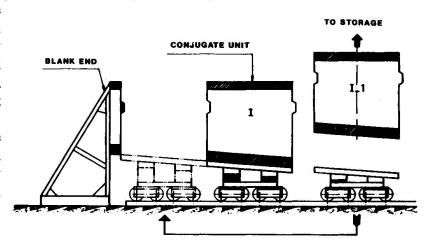
FABRICATION OF SEGMENTS Steps used in precasting operation
