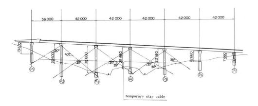
Fig. 6 Temporary stay cable arrangement
