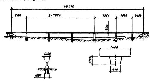
Fig. 1 Diagram of superstructure
