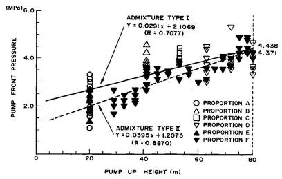
Fig.6 Transition of pump front pressure
