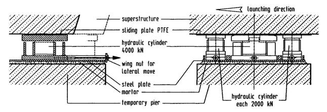
Figure 4. Launching bearing on a temporary pier
