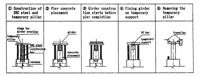
Fig. 4 Pier construction method
