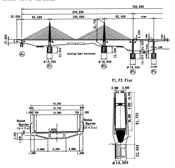
Fig. 1 Elevation and typical cross section
