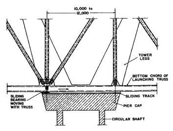
Fig. 3 Truss moving on pier table
