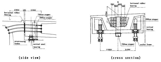
Fig. 5 Bearing at abutment
