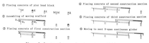
Figure-3 Construction procedure by moving scaffold
