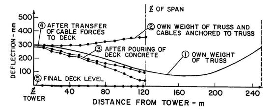
$\underline{\text{Fig.5}}$  Deflection of truss and deck during construction for temporary deck elevation + 300 mm
