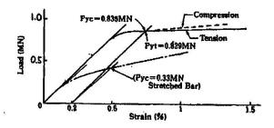
Fig.3 Load-deformation tests on the Steer-bars
