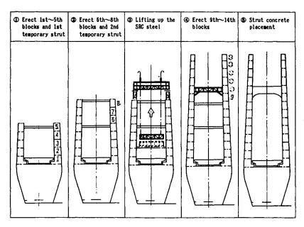
Fig. 5 Tower construction method
