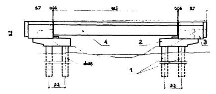
Fig. A bridge with the 16.5 m span
