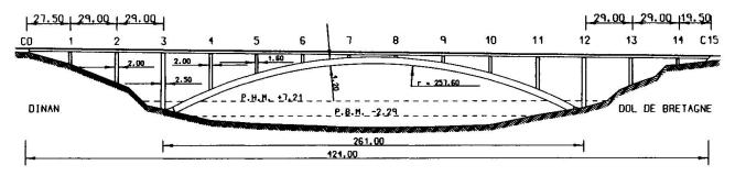
LA RANCE BRIDGE - A structure made of an high strengh concrete arch supporting a composite deck
