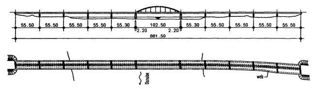
Figure 3. Elevation and plan view of structure of Danube Bridge Fischerdorf
