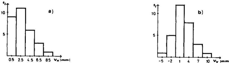
**Fig.4** Deviations of transversal beams and longitudinal stiffeners
