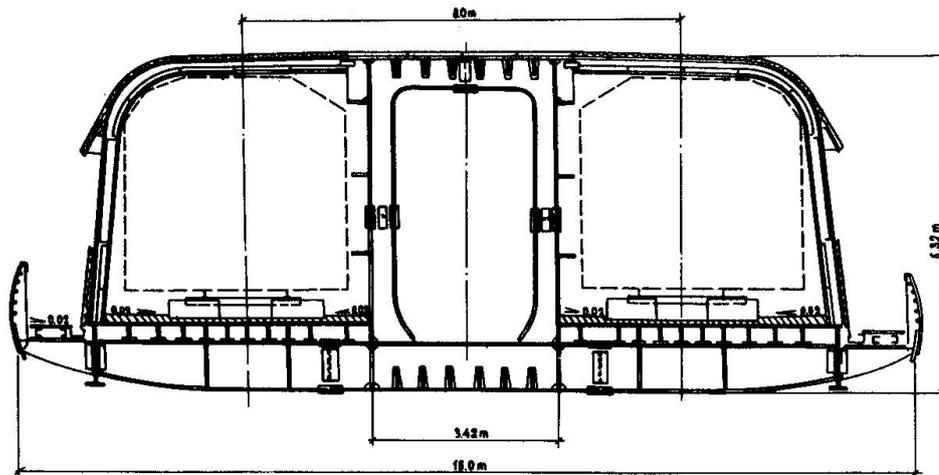
Fig. 1 Superstructure cross-section
