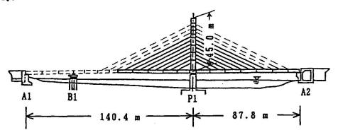
Fig. 2 Erection of Bannaguro Bridge (13th and final stages)
