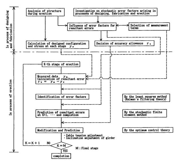
Fig. 1 Flow-chart of method for accuracy control
