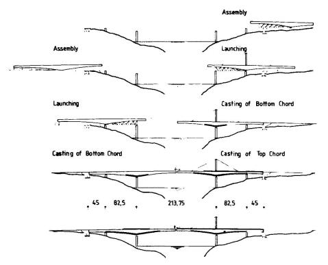
Fig. 5: General sequence of construction
