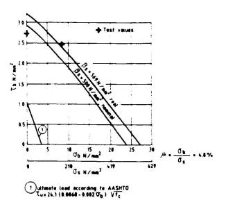
Fig. 3: Shear versus tensile strength
