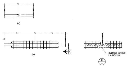
Figure 8. Peace River Bridge bottom flange details, (a) welded splice, (b) bolted splice. The contractor concurred with all of these decisions by the designers, and found them useful for the erection of the bridge.
