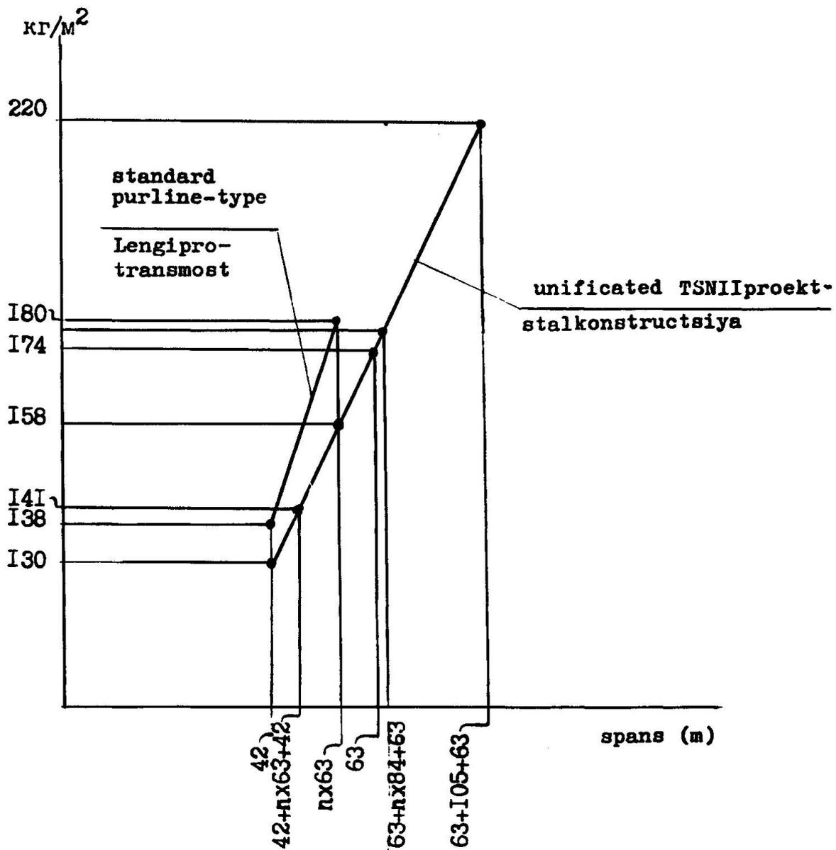
Fig.4 Metal consumption for composite superstructures.
