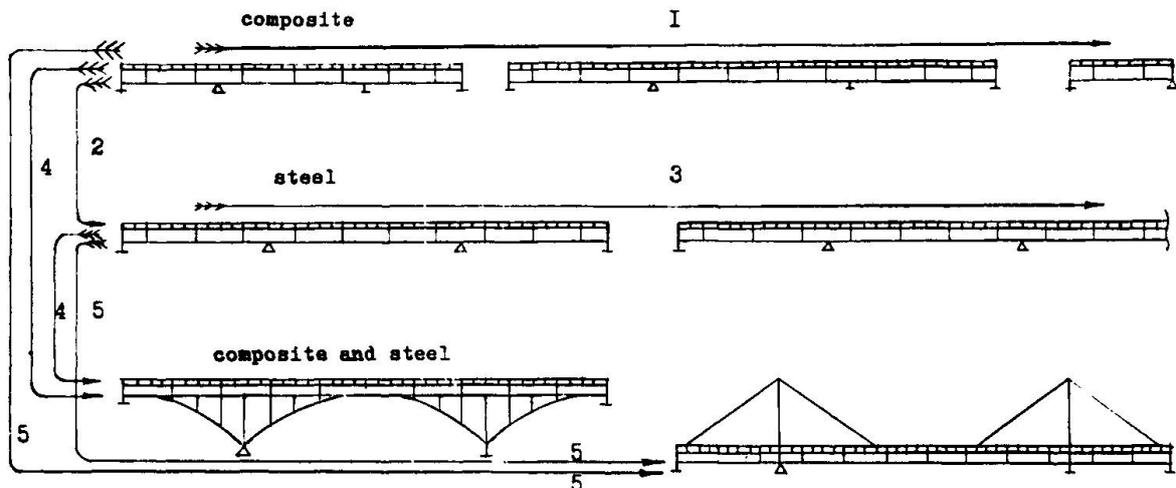
Fig.1 Unification of highway bridge superstructures with I-beams.
