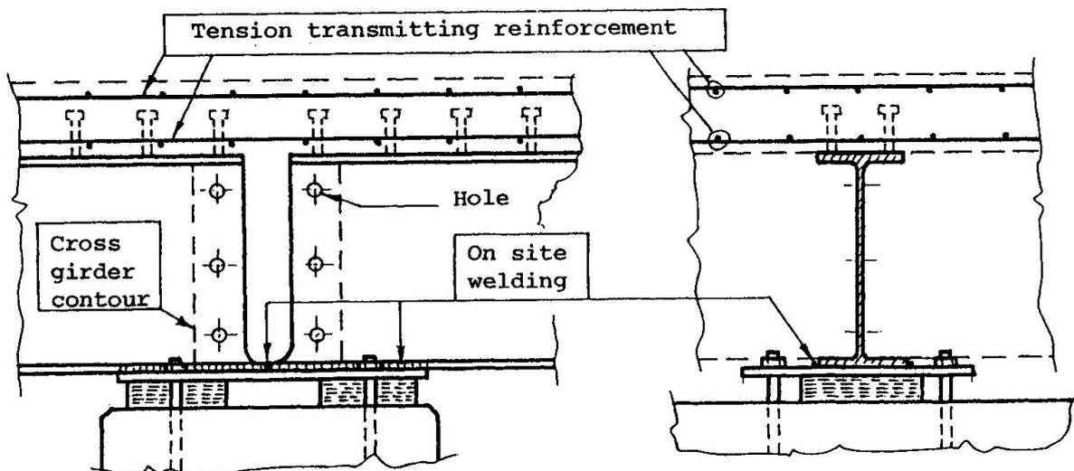
FIG. 3 Welded bottom flange connection for continuity
