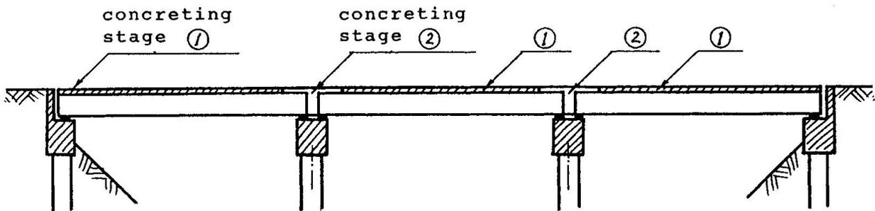
FIG. 1 Sequence of concreting the deck
