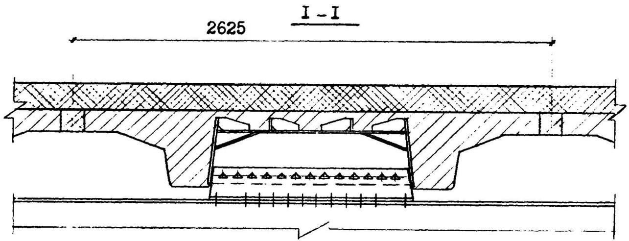
Fig.3 A r.c. slab with a steel top chord assembly.
