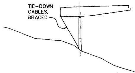
Figure 2. Carnes Creek Bridge, placement of first girder.
