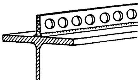
The shear transfer between the steel structure and the concrete top and bottom chord is achieved by Perfbond strips, Fig. 4; that is by continuous steel plates  $\phi$  70 x 12 with holes  $\phi$  35 mm at 50 mm. Numerous tests have shown that these strips have an ultimate capacity of about 1800 kN/m, [3].
