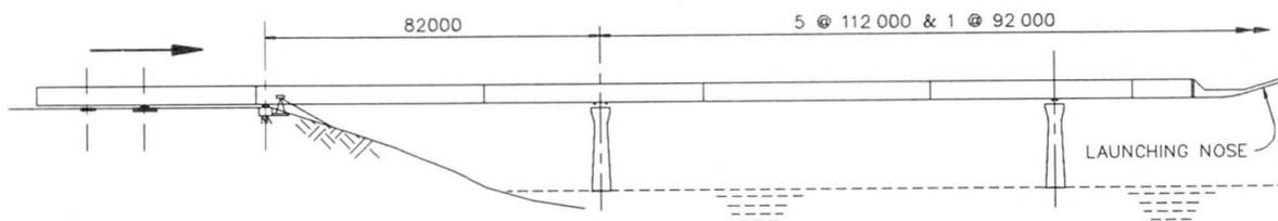
Figure 7. Peace River Bridge under construction by launching.
