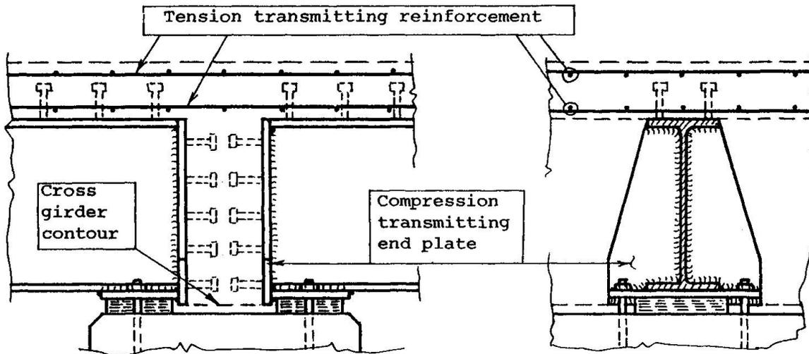
FIG. 2 End-plate type connection for continuity under Live Load.
