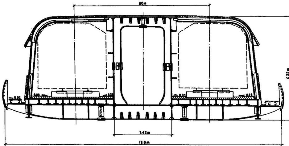
Fig. 1 Superstructure cross-section
