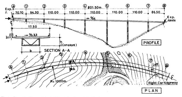
Fig.1 - Plan, Profile and Typical Deck Section of the Viaduct.
