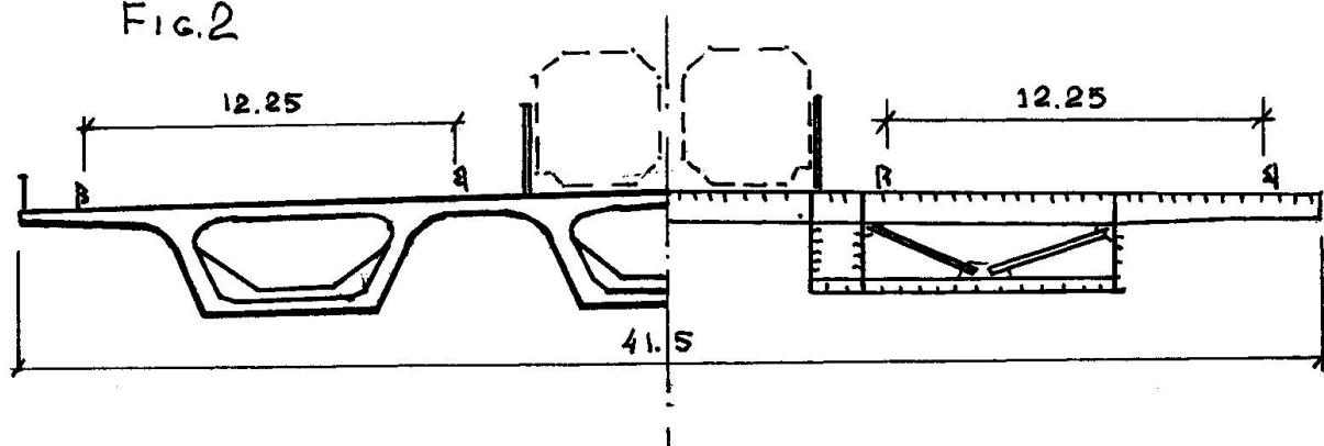
The bridge is designed to carry six motor traffic lines, two underground railway lines and communications - pipelines of large diameter. The cross section of the concrete and steel part of the bridge you can see in Fig. 2.
