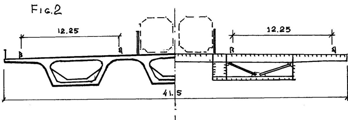
The bridge is designed to carry six motor traffic lines, two underground railway lines and communications - pipelines of large diameter. The cross section of the concrete and steel part of the bridge you can see in Fig. 2.
