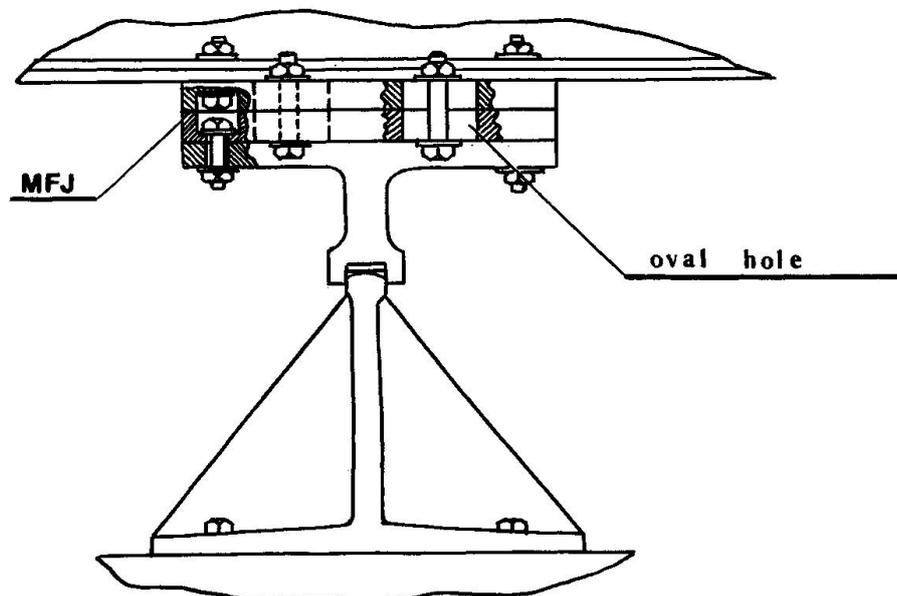
Fig.1. Construction of the supporting part with FMJ
