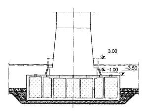
Pier caisson and pier shaft
