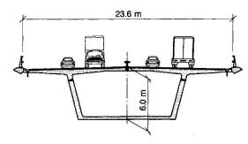
Cross section of concrete girder
