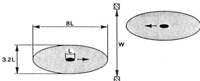
Fig. 3: Principle of the empirical rule for minimum span width assuming that vessels travel on service speed.
