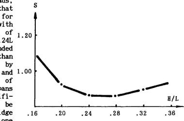
Fig.2 Cost of superstructure versus H/L
