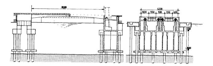
Fig. 4: Bascule Bridge, General Arrangement
