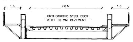
Fig. 1. Frederikssund Bridge. Rehabilitation of Bascule Span.
