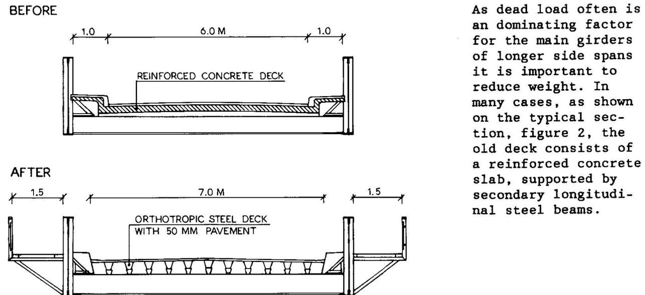
Fig. 2. Frederikssund Bridge. Rehabilitation of Side Spans.
