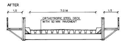
Fig. 2. Frederikssund Bridge. Rehabilitation of Side Spans.
