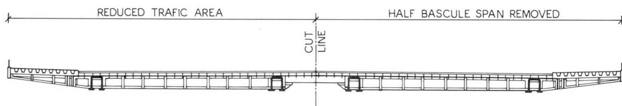
Fig. 5. Knippels Bridge. Cross Section of Bascule Span.
