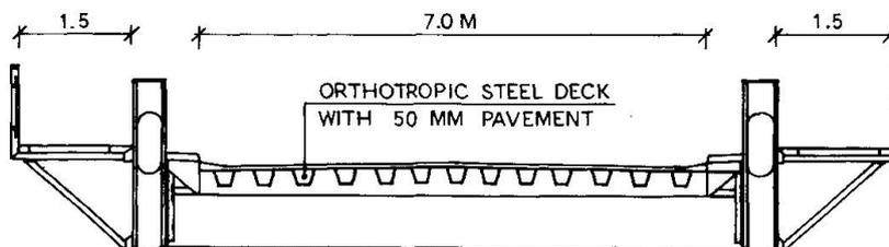
In order to save load and carrying capacity the deck including the secondary longitudinal girders was replaced by a modern orthotropic steel deck as shown in the figure. Normally the deck plate has a thickness of 12 mm and is supported by trapezoid formed ribs with a centre line distance of 30 cm.
