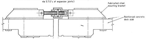
Fig. 6 Substructure Load Sharing Using STUs
