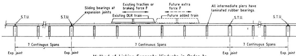
**Method of Linking Separate Viaducts in Order to Distribute Increased Longitudinal Forces**
