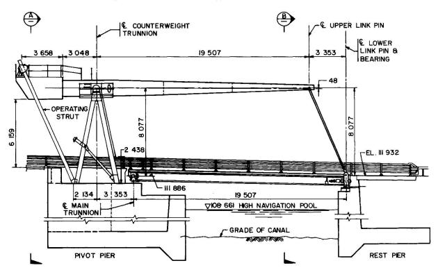
Fig. 2 Lock Street Bridge Replacement-South Elevation
