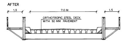
Fig. 2. Frederikssund Bridge. Rehabilitation of Side Spans.
