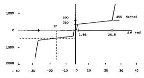
$\frac{\text{fig.4}}{\text{C}_1}$  Moment-rotation characteristic of  $\text{C}_1$  in fig.3
