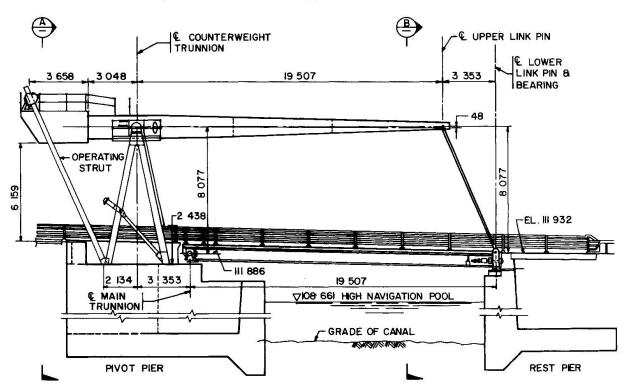
Fig. 2 Lock Street Bridge Replacement-South Elevation
