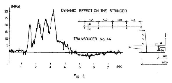
Dynamic measurements are illustrated by Fig. 3. Analysis of measured strains on stringers at a train velocity of 60 km/h resulted appr.15% stress increase because of dynamic effect.
