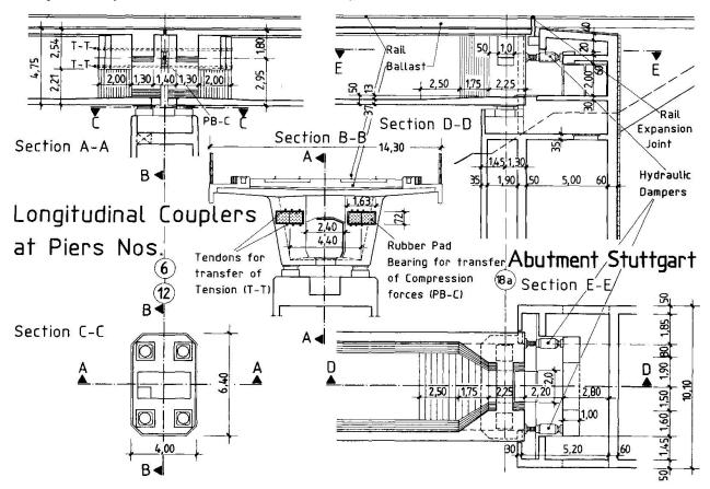
Enz-Viaduct: Coupling devices, hydraulic dampers and rail expansion joint
