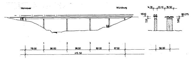
Fig. 7 Werra Viaducts: Elevation and cross-section
