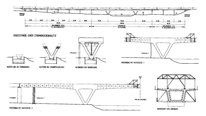
Fig. 4 Viaduct near Gemünden: Overall view and construction
