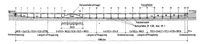
Fig. 5 Viaduct near Veitshöchheim: Elevation view
