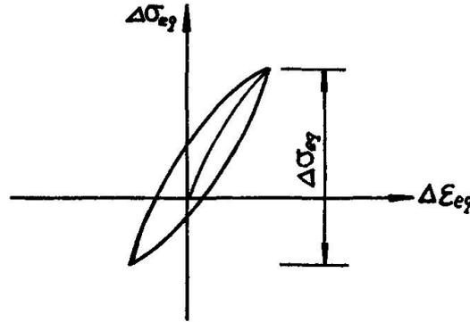
**Fig.1** Stress-Strain Cycle
