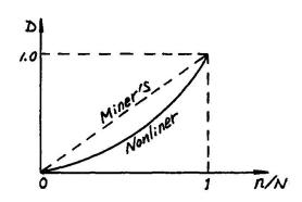
Fig. 2 Fatigue Damage Accumulating
