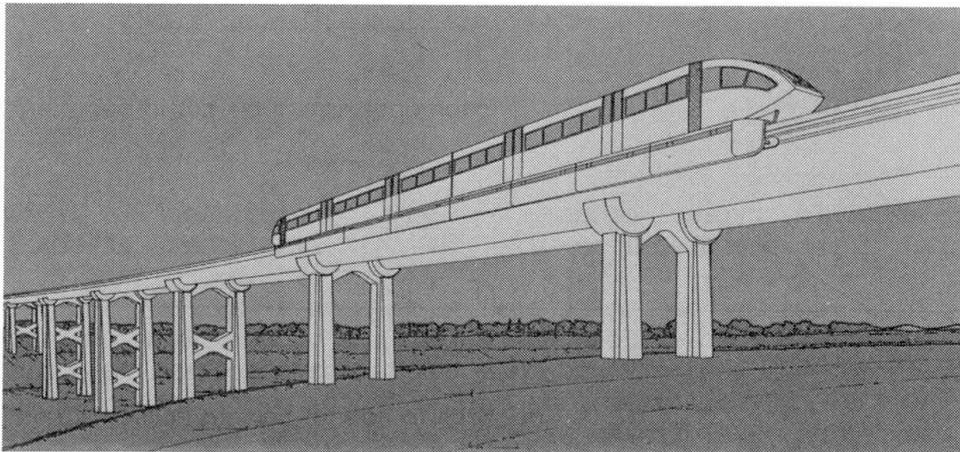
Fig. 5 Elevated double-track guideway, drawing in perspective
