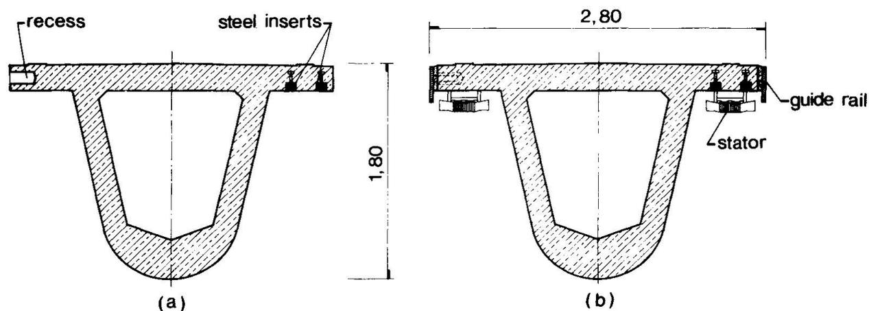
Fig. 2 Girder cross section TVE, 2nd construction phase
