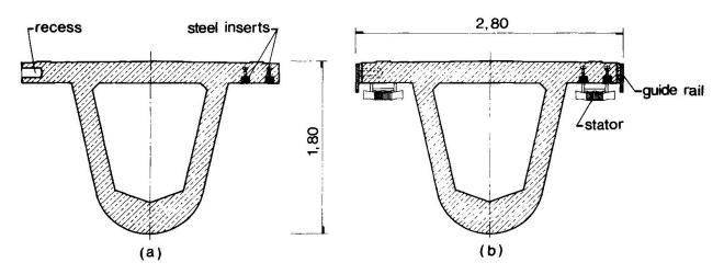
Fig. 2 Girder cross section TVE, 2nd construction phase
