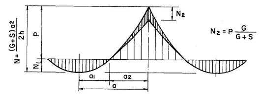
Fig. 5 Axial forces in deck with prestress
