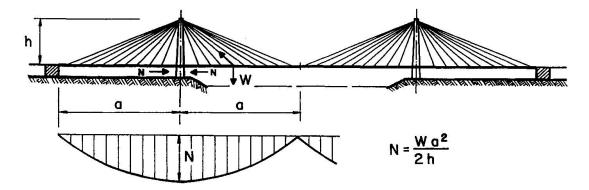
Fig. 1 Generalized cable-stayed bridge schematic
