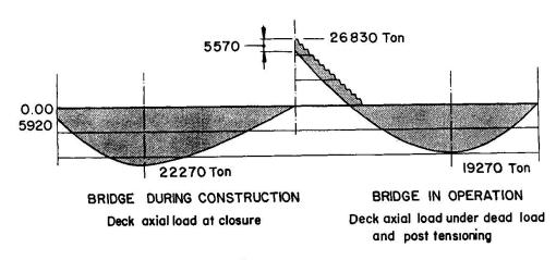
Fig. 8 Axial forces in deck during construction
