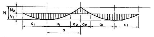
Fig. 4 Axial forces in deck without prestress
