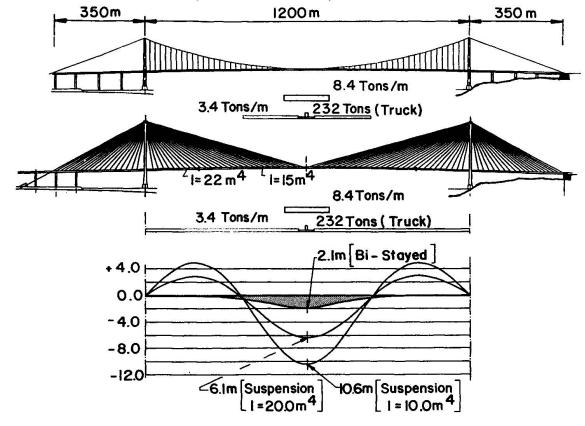
Fig. 6 Comparison of deformational characteristics
