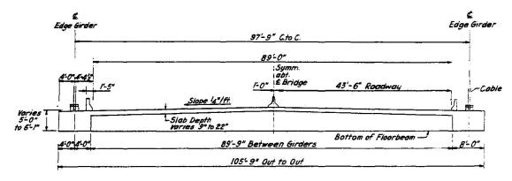
FIGURE 2 - CROSS SECTION
