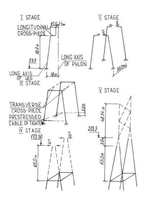
Fig. 3 Pylon erection diagrams
