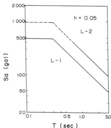
Fig.10 Acceleration response spectra on the base stratum
