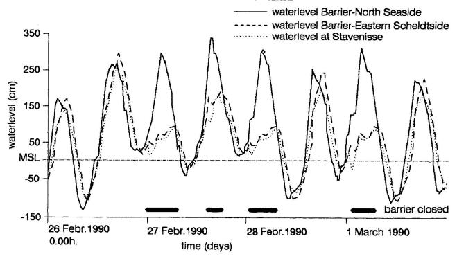
Fig. 2 Water Levels in the Eastern Scheldt during storm-surges.
