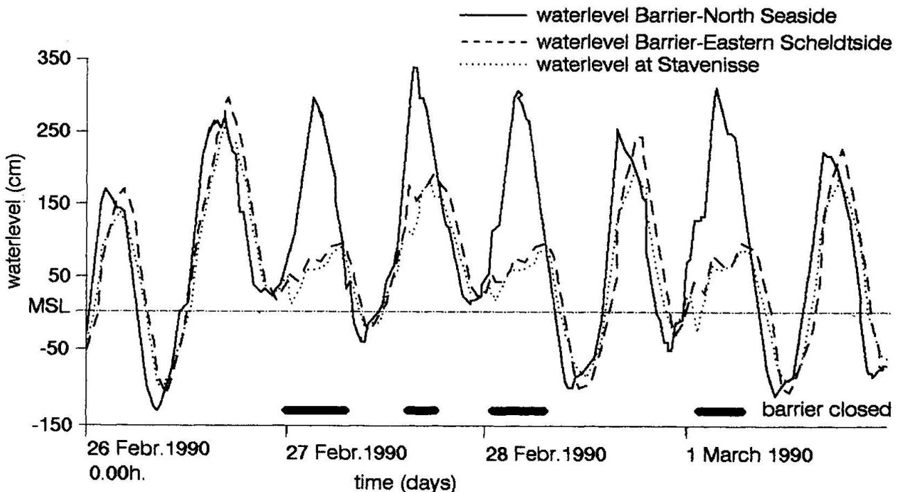
Fig.2 Water Levels in the Eastern Scheldt during storm-surges.
