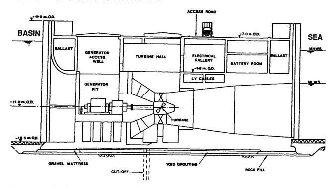
Figure 3 - Turbine-generator caisson
