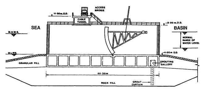
Figure 4 - Sluice caisson
