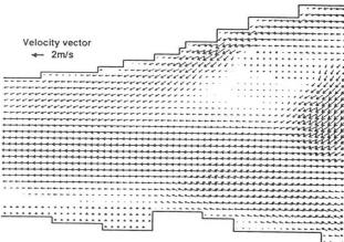
Figure 8 Tidal Streams without Barrage
