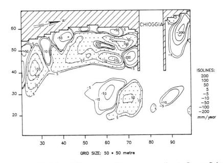
Fig. 11. Calculated Initial Bed Level Changes per Year corresponding to Strong Scirocco Wind.
