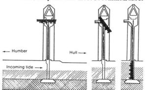
Fig. 3a: HULL lifting storm surge barrier.
