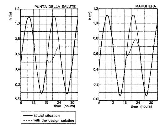
Fig. 5 Effects of the designed solution on tide level at Punta della Salute (Venice) and Marghera.
