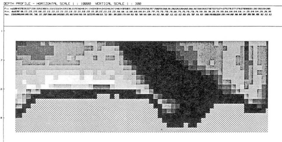
During Plume tracings a number of water samples are gathered for suspended sediment analysis over a wide dB range in order to establish a calibration curve between the back-scattered signals strength and concentration
