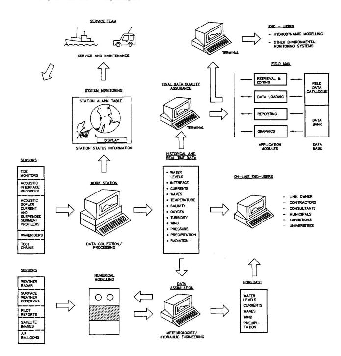
Fig. 2 Hydrographic Information System Setup.
