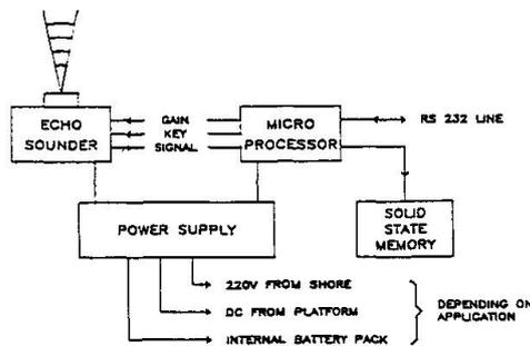
In this instrumentation setup the Acoustic Interface Recorder is incorporated in seven deployed sea bed stations and one on the survey vessel.
